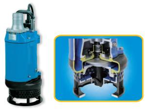
**NEW** Tsurumi Agitator Pump **KTD Series** is a cast iron made, heavy-duty slurry pump employing the KTZ Series as the base. An agitator is provided to assist smooth suction of the pumping fluid. The side-flow, top-discharge design keeps the motor cooling even if the pump is operated continuously with its motor exposed in air, and it makes the pump easier to place in a confined space.
