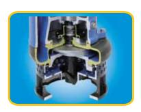
**TSURUM** Agitator Pump **KTD Series** is a cast iron made, heavy-duty slurry pump employing the KTZ Series as the base. An agitator is provided to assist smooth suction of the pumping fluid. The top-discharge design keeps the motor cool, even if the pump is operated continuously with its motor exposed in air, and it makes the pump easier to place in a confined space.
