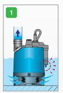
Pump continues to run while e-probe remains submerged.
