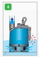
When water level rises back up and reaches the e-probe, pump resumes operation.
