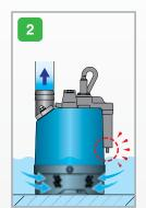
When water surface falls below the e-probe, timer begins a 1-minute countdown.
