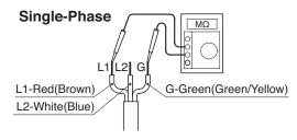
**Note:** The insulation resistance reference value of 20M  $\Omega$  minimum is based on a new or repaired pump. For reference values of a pump that has already been put into operation, refer to "7. Maintenance and Inspection" of
